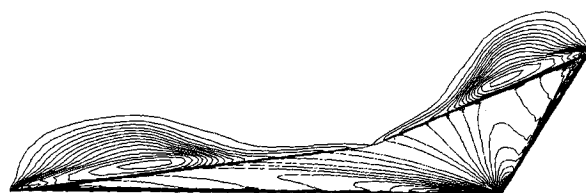
Fig. 4 Carlson arrow wing, M_\infty = 2.05 , \alpha = 8 deg, total pressure loss isolines.
